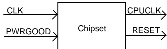
Figure 2. Internal Delay Function of Chipset
