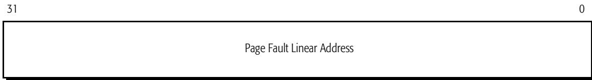
Figure 21. Control Register 2 (CR2)
