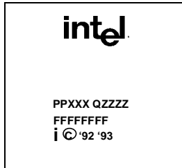
mcC0-Step Engineering Sample TCP Units:
