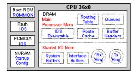
The 3600 Series Routers are particle—based platforms. The interface buffers are atomic buffers, called particles, into which the packets are split. When a packet cannot be fast—switched, the router has to reassemble it in one system buffer because the process switching code cannot handle particles. Public particle pools cannot be tuned.
